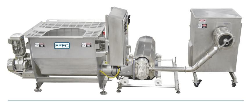
•40 HP MOTOR WITH OPTIONAL FREQUENCY CONTROLLER FOR EXACT KNIFE RPM SETTINGS
